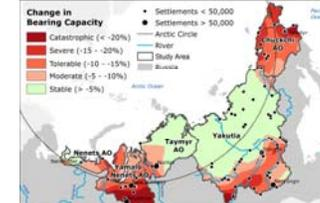
Figure 6. Temporal changes in foundation bearing capacity between the 1970 and the 2000 periods.
