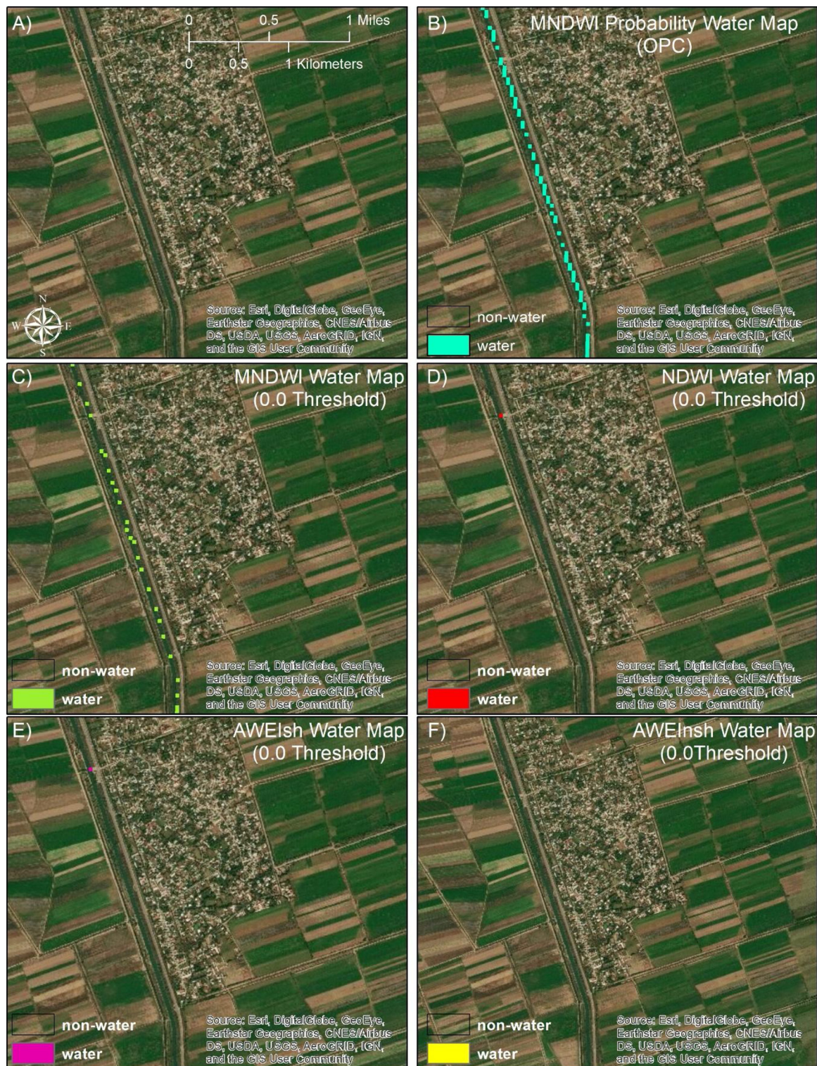
Fig. 8. Compares the ability to detect the Upper Garabakh Canal, Azerbaijan, between the selected water indices and the MNDWI probability water map, using the OPC method. A threshold value of 0 was applied to each water index. (A) Shows a true-color image of the Upper Garabakh Canal. (B) Canal water detected by the MNDWI probability water map. (C) Canal water identified by MNDWI water index (D) Canal water identified by the NDWI water index (E) Canal water detected by the AWEIsh water index. (F) Canal water identified by the AWEInsh water index.
