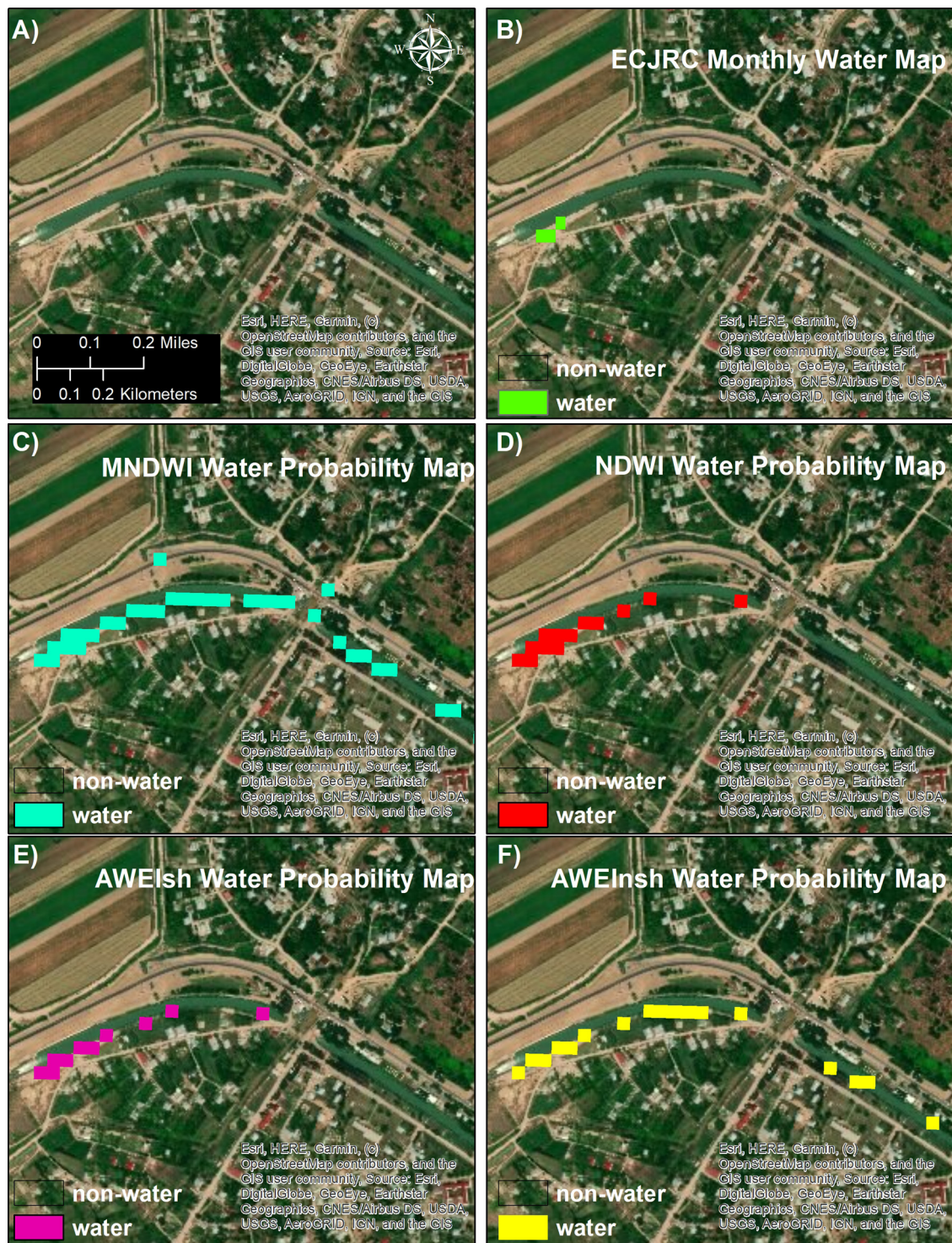
Fig. 3. This figure displays the difference in water detection ability based on the OPC maps of a canal just East of the city of Agjabedi, Azerbaijan. (A) displays the water canal in Agjabedi, Azerbaijan. (B) the ECJRC Monthly History water map. (C) MNDWI water probability map. (D) NDWI water probability map. (E) AWEIsh water probability map. (F) AWEInsh water probability map.
