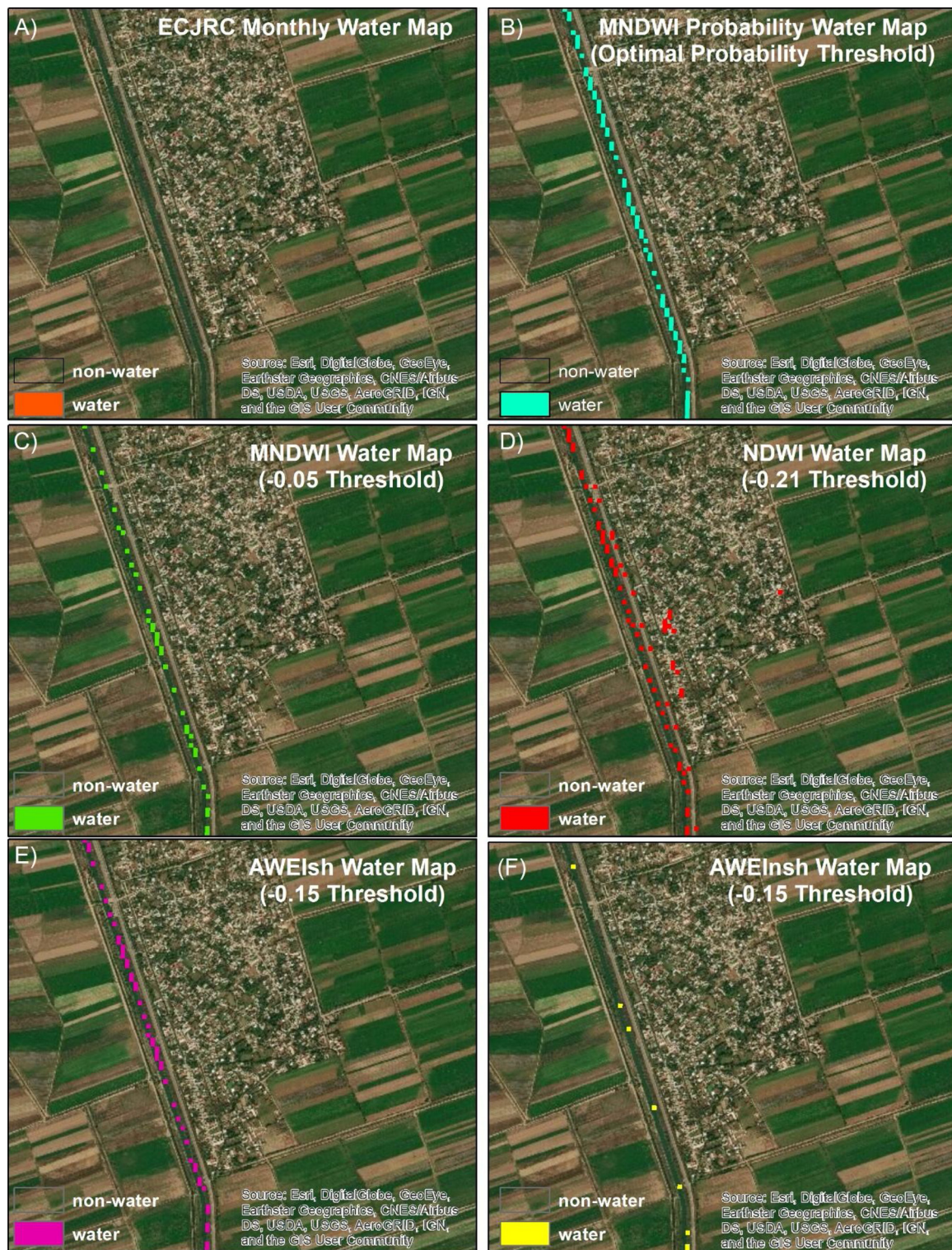
Fig. 9. Compares the ability to detect the Upper Garabakh Canal, Azerbaijan, between the selected water indices, the ECJRC Monthly History water map, and the MNDWI probability water map, using the OPC value method. The thresholds chosen for the selected water indices were determined by applying the lowest potential threshold value for each water index, as listed from previous studies. (A) shows a true-color image of the Upper Garabakh Canal. (B) Canal water detected by the MNDWI probability water map. (C) Canal water identified by the MNDWI water index (-0.05 threshold). (D) Canal water identified by the NDWI water index (-0.19 threshold). (E) Canal water detected by the AWEIsh water index (-0.15 threshold). (F) Canal water identified by the AWEIsh water index (-0.15 threshold).
