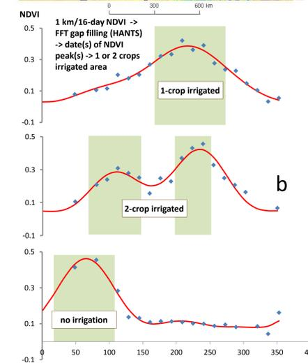
Fig. 6. Land surface phenology analysis: (a) NDVI on irrigated lands in late summer in central Asia, (b) original 16-day NDVI filtered values (blue dots) using Fourier Fast Transform (HANTS approach) (red line) and extracted the dates of NDVI peaks (green bars). Timing and number of NDVI peaks provide crucial link for identification of irrigated lands, because in the semi-arid and arid climate of central Asia non-irrigated vegetation rapidly decline after short spring greening.
