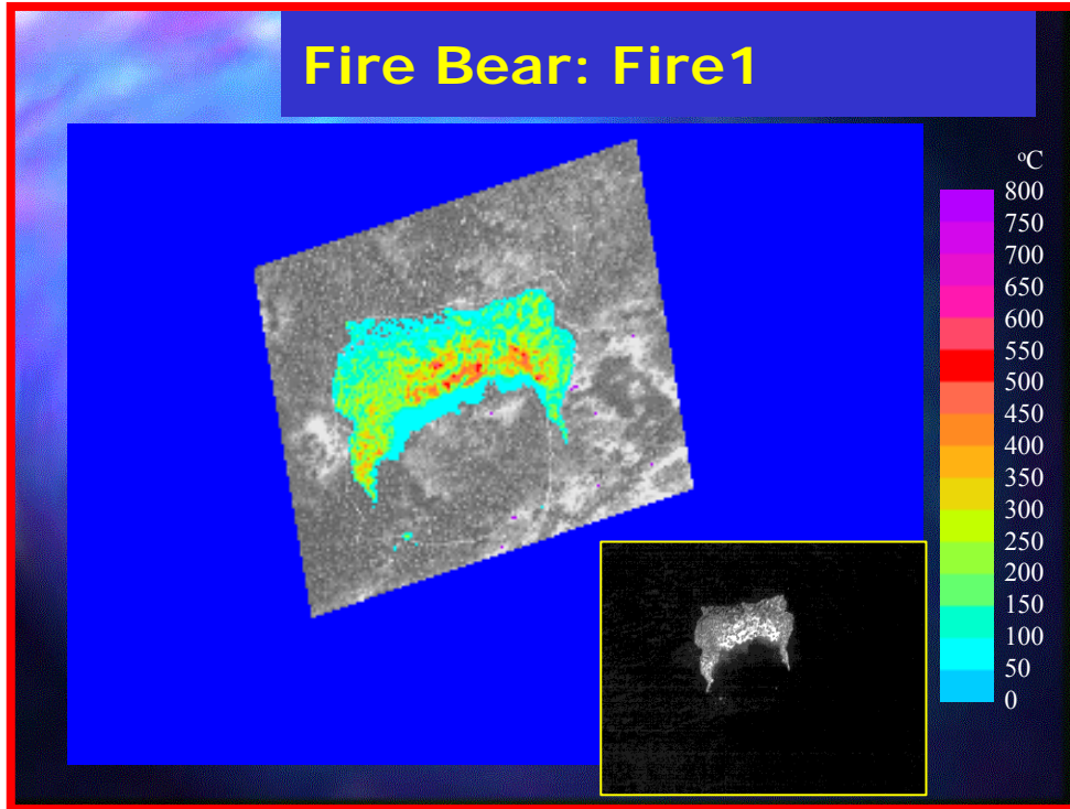
Figure 10. Aerial infrared images, taken during the experimental fires, were analyzed to quantify fire behavior parameters (e.g., rates of spread, fire temperatures, reaction intensity, etc.) that can characterize fire severity.
