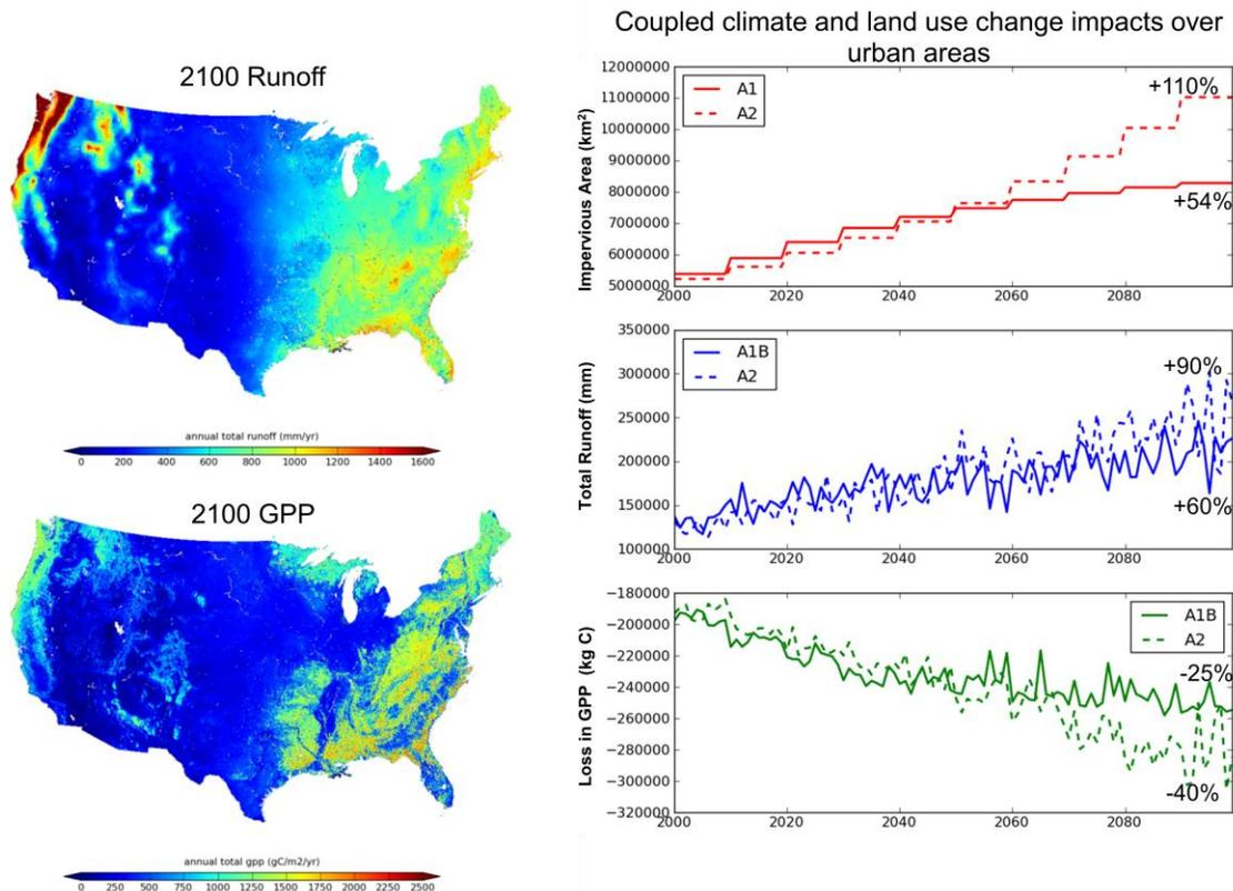
Figure 3. Sample results from the coupled climate and land use change model runs, showing predicted patterns in annual runoff and GPP for the U.S. at 1km resolution (left), along with the predicted changes in impervious surface area, runoff, and gross primary productivity for urban areas from 2000 to 2100 under the SRES A1B and A2 climate scenarios (right).
