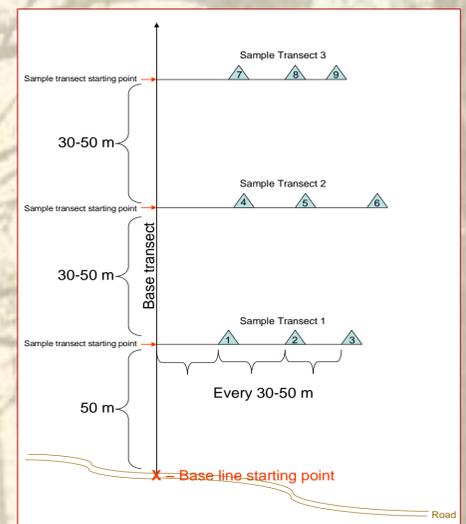
Fig.8. The basic sampling layout, showing base transect, sample transect, and sample triangle locations used to characterize one unit.
