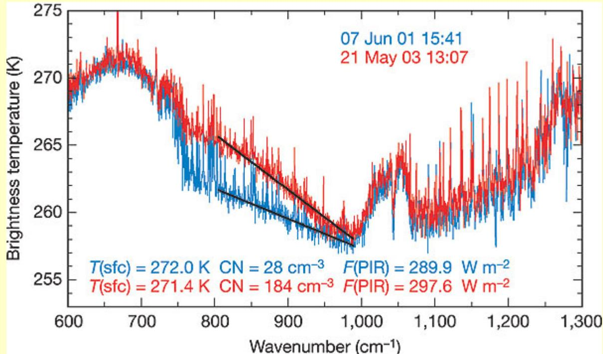
Downwelling emission spectra measured by the NSA AERI beneath two clouds with very different condensation nuclei (CN) concentrations.
